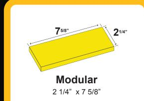
Brick Type: Modular Size: 7.625" x 2.25" Tolerance: +0", -1/16"
