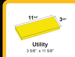
Brick Type: Utility Size: 11.625" x 3.25" Tolerance: +0", -1/16"
