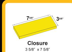
Brick Type: Closure Size: 7.625" x 3.625" Tolerance: +0", -1/16"
