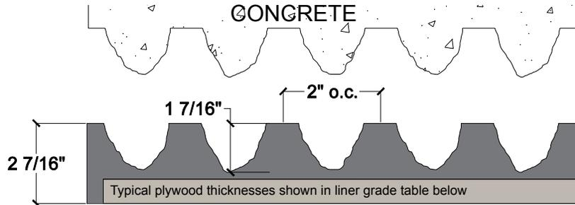
*\*Typical liner thickness shown. Final thickness will be determined on a per job basis.*
